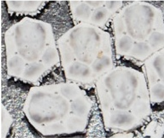
Fig. 4 – Osteoderm after heating in a furnace to 550 °C for 24 h. The organic substance and water were baked off, leaving only the mineral phase.
